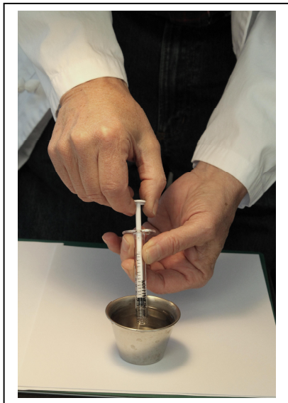
Method 1: Immerse the tip of syringe directly and fill it prior to attaching the MicroSprayer® Aerosolizer
