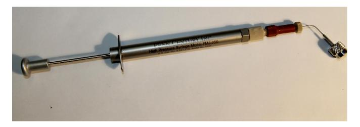
The Penn-Century MicroSprayer<sup>®</sup> Aerosolizer – Model IA-1C is a unique, air-free atomizer. It generates an aerosol when liquids, solutions or particle suspensions are pushed at high manual pressure through tiny patented aerosolizing components in the tip of the device.
