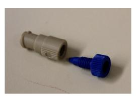
– that is, *in reverse* direction from tip to the hub. Although this tool may not help in every case, in most cases, when correct procedure is followed, this process will loosen and force out whatever is blocking (clogging) the tip of the MicroSprayer® and return it to good working condition.
