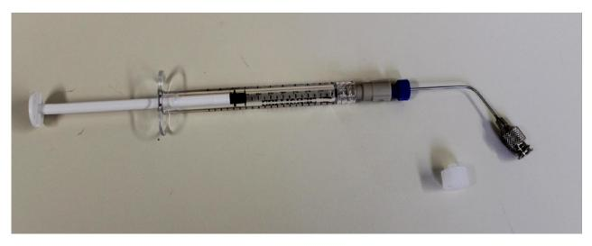
The Penn-Century MicroSprayer® Aerosolizer – Model IA-1B is a unique, air-free atomizer. It generates an aerosol when liquids, solutions or particle suspensions are pushed at high manual pressure through tiny patented aerosolizing components in the tip of the device.
