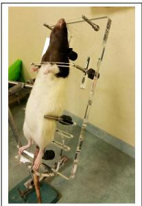
The Intubation Platform for Rat (IPR) by Penn-Century is designed to make intubation of anesthetized rat faster, safer and easier.
